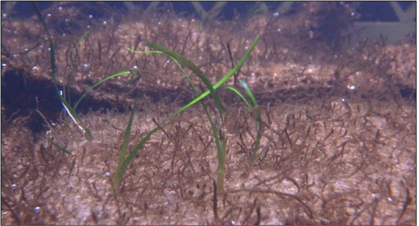
Figure 4. The laboratory trial hessian, once degraded, and the emergent Z. marina plants. Photo by Emma Nolan.
