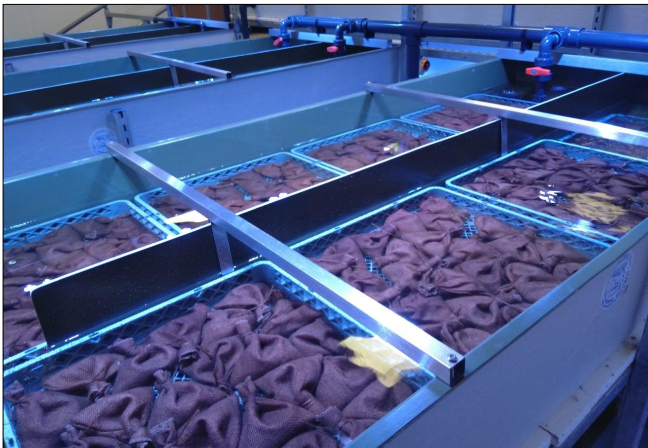
Figure 3. The laboratory trial hessian bags containing 30 seagrass seeds and/or seedlings amidst a sand/loam mix. Photo by Emma Nolan
