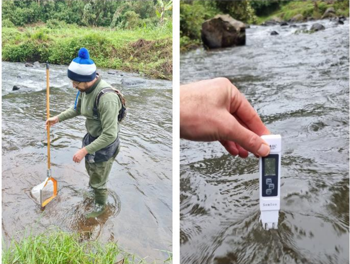
Fig. 8: Kick-sampling a site (left) and taking measurements of electrical conductivity (right).
