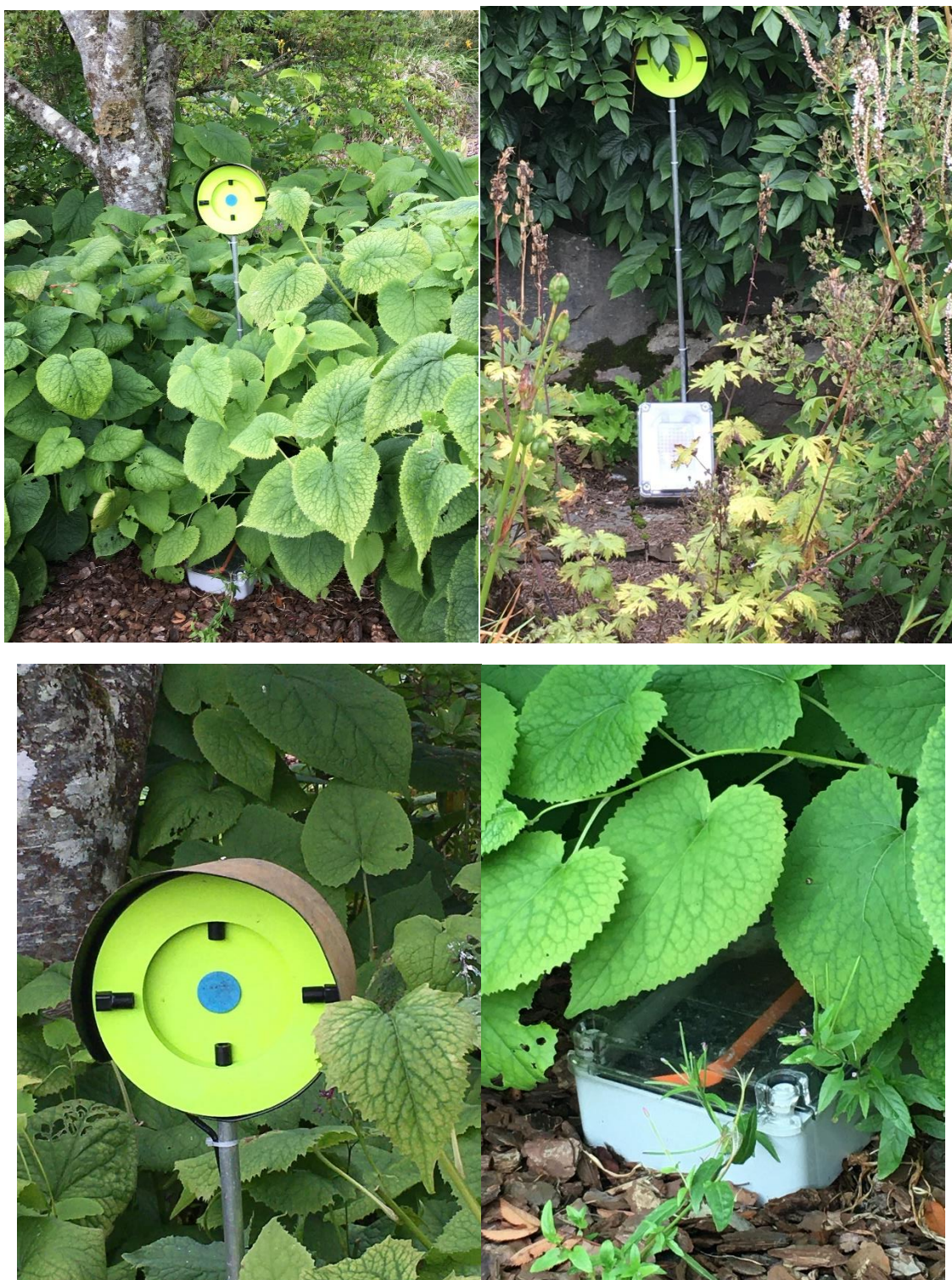
Figure 8.11. 1 'POLY' an automatic in-field sensor for Pollinator surveys at Inverewe gardens, Poolewe, Wester Ross. In collaboration with National Trust for Scotland, AgriSound and Innovate UK (AgriSound, 2021).
