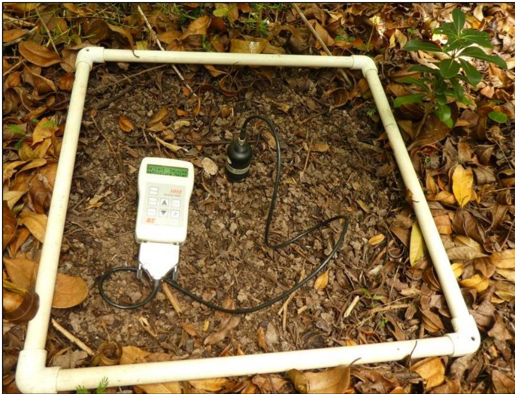
Figure 3: Soil Moisture sensor in snail quadrat cleared of leaf litter at random site 16.
